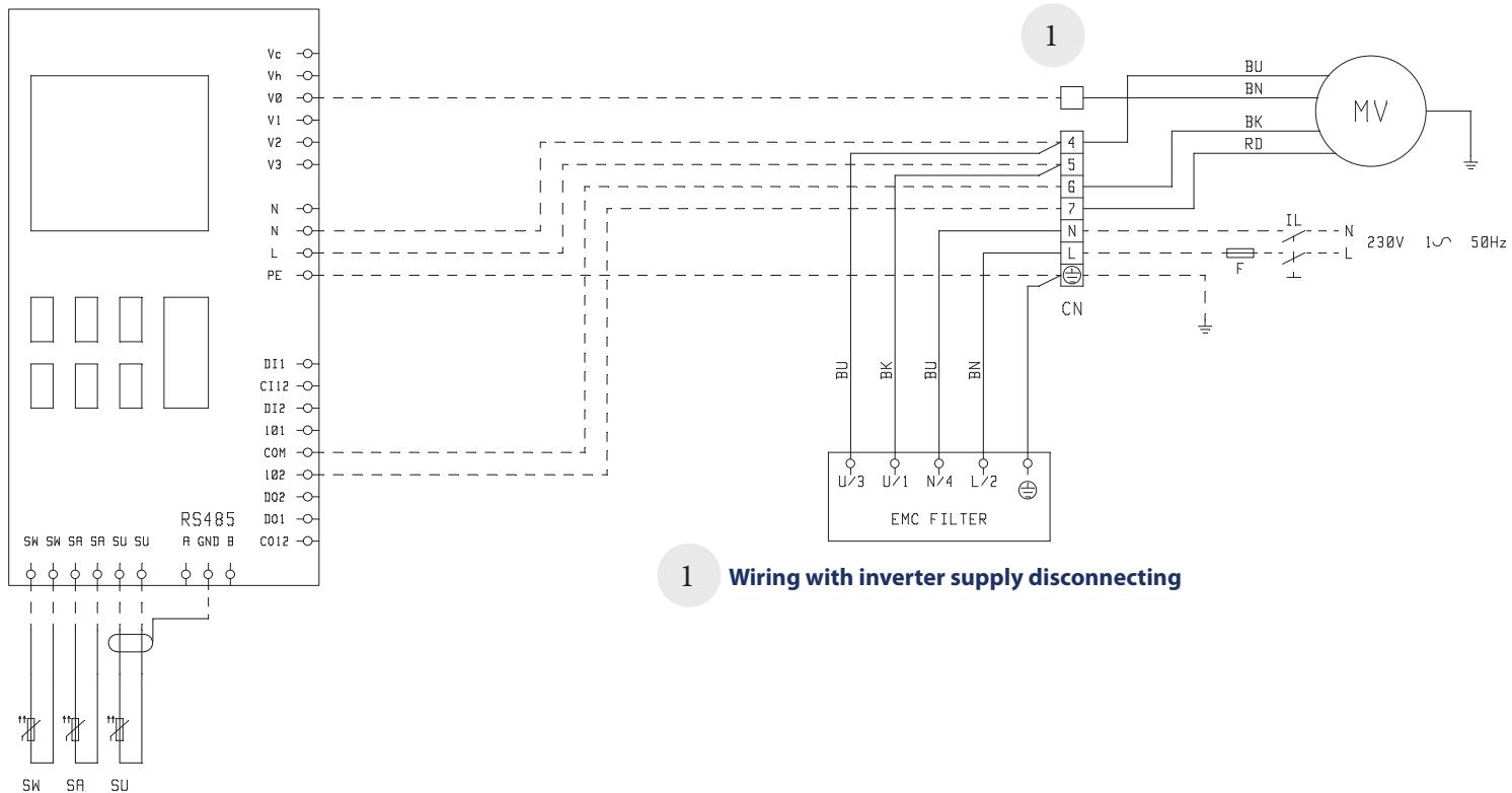
1 Wiring with inverter supply disconnecting
